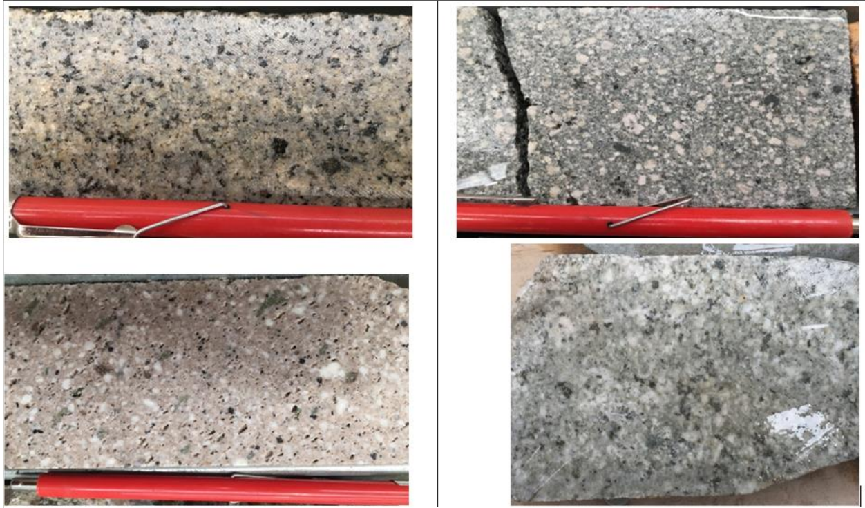
Figure 7.5: Top Left, LAV-064 (400 m) - Crowded Porphyritic Dacite Top Right, LAV-117 (218 m) - Granodiorite, Bottom Bottom Left, LAV-114 (40.5 m) Tonalite Bottom Right, V2017-04 (442.5 m) Granodiorite Porphyry
