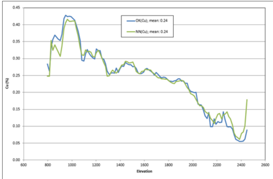
Figure 14.37: Elevation – Ordinary Kriging vs Nearest Neighbour for Copper
